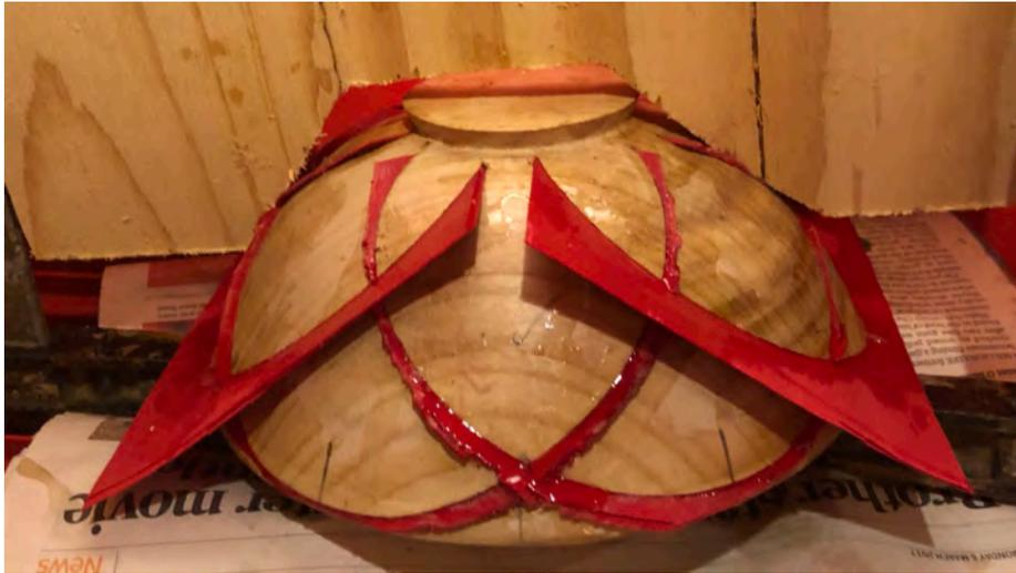
The piece on the bandsaw jig is above, and a gluing and clamping stage below (three stages are needed because of the intersections). The clamping was done because the kerfs can open a little (unlike in the previous case) and clamping them down helps. It is not clear what else could be done short of cutting right through and gluing conventionally.
