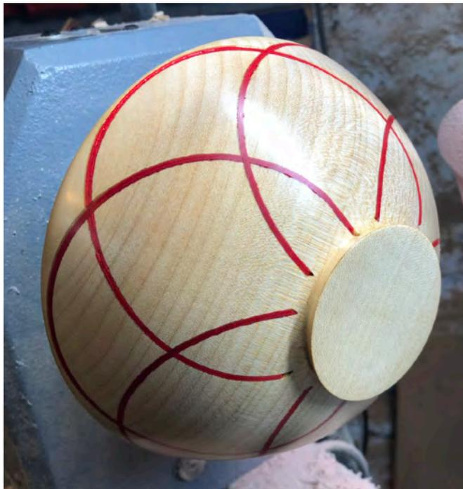
The wood is sycamore, the central (padauk) boss is made separately and glued into a shallow hole in the bowl centre made on the lathe using a Forstner bit.
