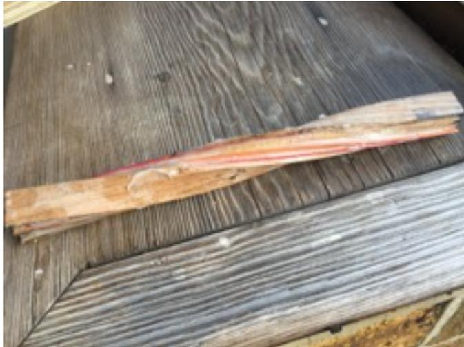
will need clamping during the gluing process, I used small G clamps at about 40mm intervals for the set above, clearly at rotating positions round the stack. The gluing process tends to be messy - I have not found out how to do this without getting one's hands covered in glue! The twisted pieces are coated and placed together in order one-by-one. Simple but a bit awkward to do.
