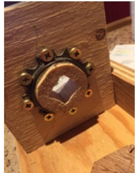
Where construction is of softwood ply with a pair of lowish cost (£7) cycle freewheel units (Diamondback DBX160 Freewheel 16T M30) with round-to-square wooden inserts glued in and screwed to holes cut in the ply, facing one another and thus with opposite ratchets. Clearly the ratchets are the point, so that the twisted wood is prevented in a simple and accurate way from untwisting. I have tried the same idea with clamps but it is very tricky!
