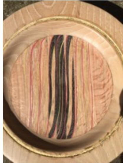
This is a technique used to make some twisted-wood items such as the candlestick stems and (unfinished) plate above, the latter being composed of nine twisted oak sets of 3\*20mm strips squared off, glued into a plank and turned. In both cases the sets include contrasting woods and/or commercial dyed veneer layers (standard thickness) for effect.
