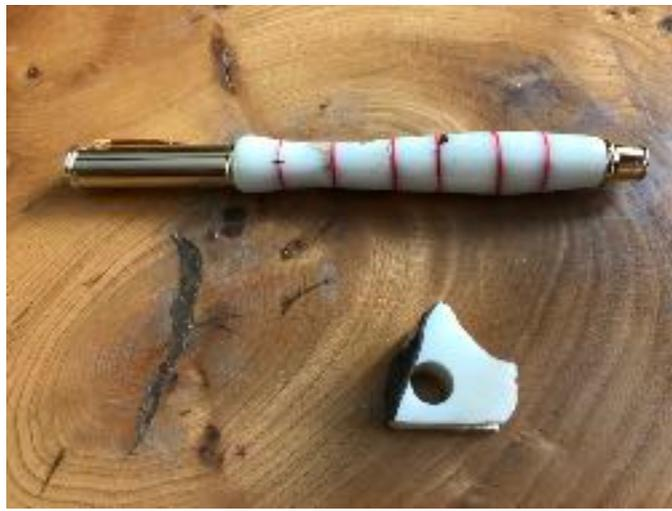
A slightly less-successful use in a pen - by slicing the nut with a bandsaw and cutting out and drilling sections (one shown below) that are then glued in a stack around a 7mm brass tube. These are then finished together as a pen barrel (in this case I have glued red veneer layers between the nut sections). Defects show but perhaps look 'natural'.
