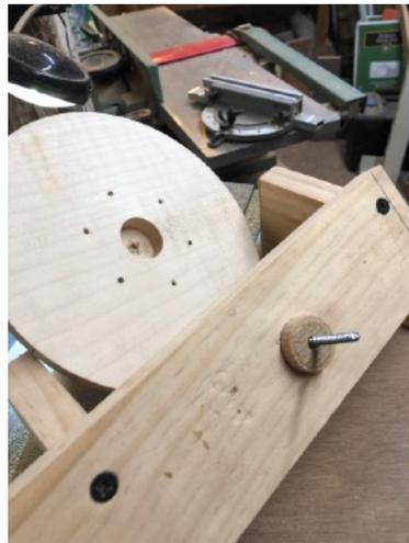
The exact jig angles in both directions are a matter of visual preference (set in this case by the jig wood components), though of course the top and bottom of the kerf should be near the base centre and rim. I might make them more angled to get a steeper spiral next time. The cut is very gently done to keep the bandsaw blade straight.
