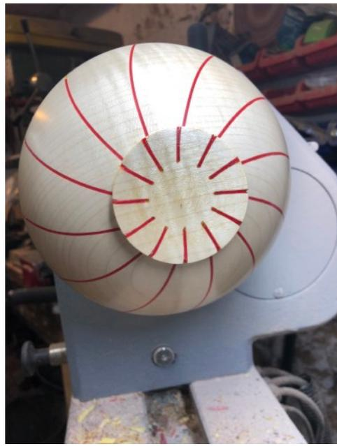
120 grit stiff abrasive paper - simple but tedious. A new bandsaw blade or a different veneer might give the correct width as sawn. The kerf reaches in a maximum of 12mm or so (see picture above).
