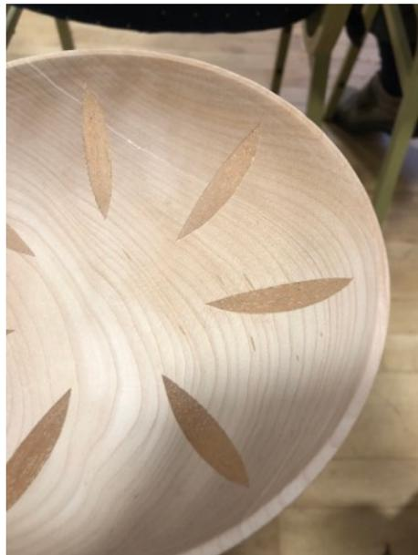
Not having a suitable router jig I used a home-made wooden jig on a bandsaw to make angled (but obviously straight/planar) kerfs, which give gentle spiral shapes on intersection with the curved bowl surfaces. The resulting bowl (165mm diameter, 70mm deep and about 5mm thick) and technique looked to me interesting enough to share. The manufacturing stages are:-
