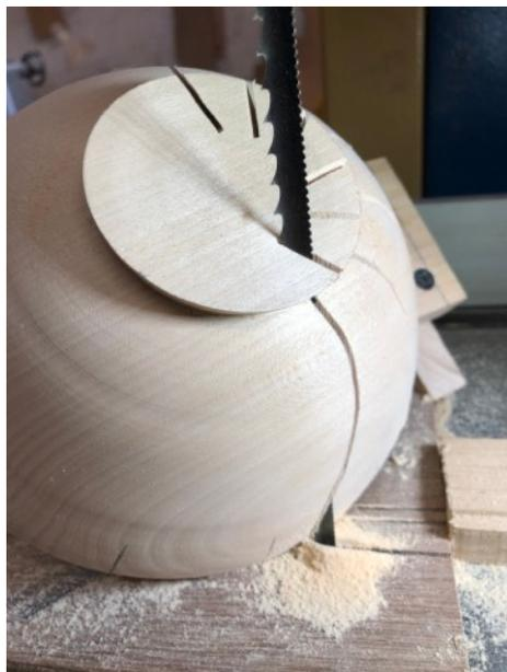
On the downside the two stage process for the two spirals (partly because it was not originally planned!) takes more off the outside of the bowl so the inside exposed veneer sections are rather short, even though the bowl is only about 4mm thick. But the concept is there. And some small pieces pulled out from the foot edge with the second bandsaw cut - possibly because the epoxy is not so strong.
