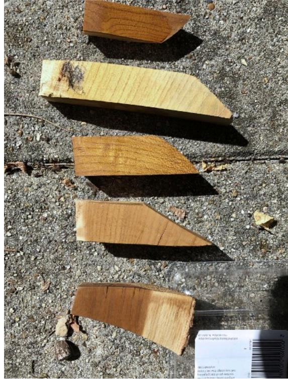
Status after another 8 days of daylight (right - previous on left). The colour of the unexposed sample in the right picture is matched to itself in the left picture with Photoshop - the real samples look a bit more brightly coloured in sunlight. They are in top-to-bottom order:-
