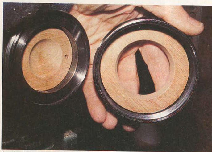
Jig for holding egg shaped objects inside combination chuck.
