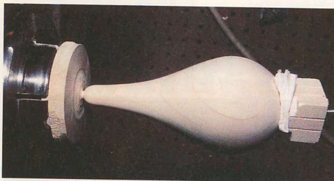
Body shape completed prior to parting off.
