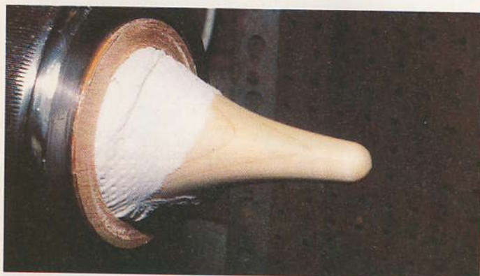
Body reversed in turning jig for finishing the tail.
