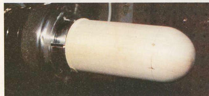
Body shaped for bird breast and leg holes marked.
