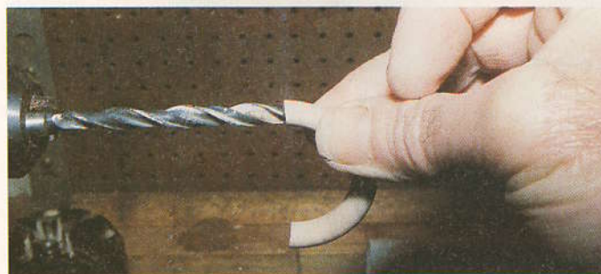
Initial concavity formed with 1/4in. drill.
