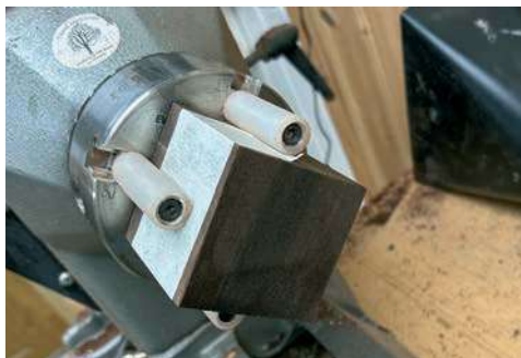
Cube box in long jaws on lathe for hollowing
