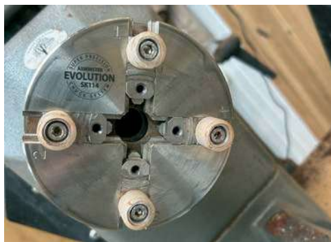
Small button jaws can be mounted in either threaded hole in jaw carrier
